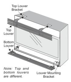
3) Open the bottom louver. Pull the Burner ON/ OFF control box from inside the bottom of the fireplace. Using the 2 screws on the louver, secure the control box in place.
